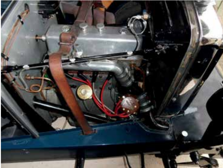
The 1/4 inch diameter, linking pipe between manifolds, is a tight fit around the Vertex Magneto.
